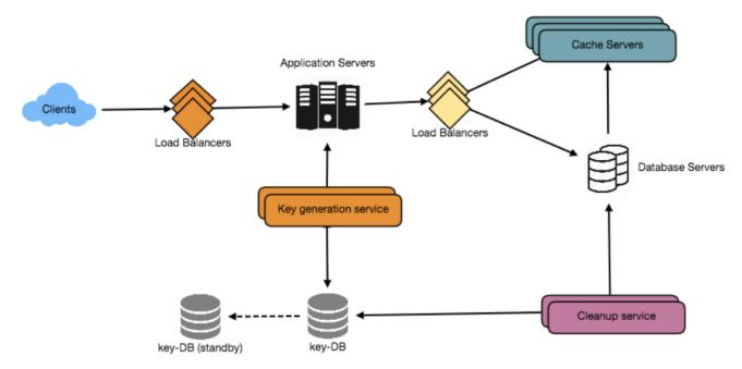
Figure 1: Detailed component design for URL shortening
